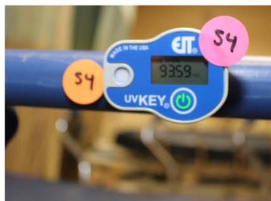
The EIT UVKey can be used to easily confirm the numerical dose value of UVC in an operating room (left) and in high touch patient areas such as a bed rail (above)
